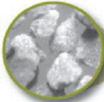
Nutshell Media Particle Size: 20–30 mesh
