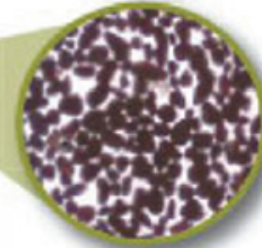
Spectrum Micro Media Particle Size: 30–230 mesh
