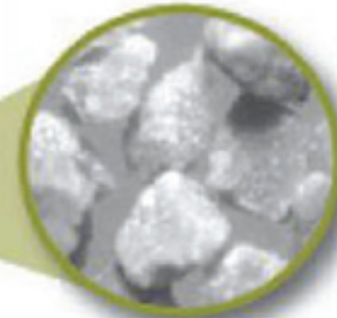
Nutshell Media* Particle Size: 20–30 mesh
